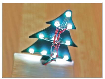
After testing the LEDs on the breadboard, I soldered 'em up into a tree. I thought this would be the hardest part, but it wasn't so tricky.
